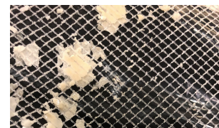
Figure 1: Example of mesh feed spacer fouling
