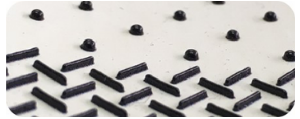
Figure 2: Printed spacers on an industry-standard membrane
